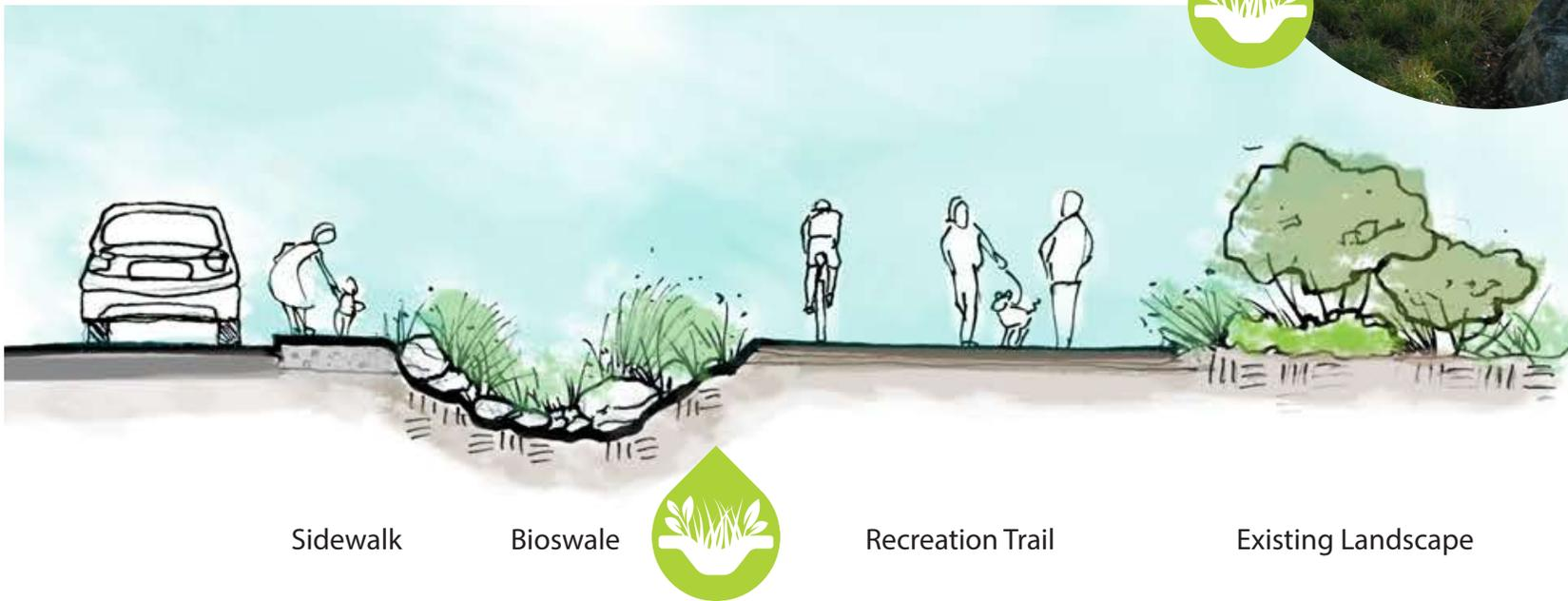
*Runoff from impervious surfaces like roads, sidewalks, and trails can be directed into bioswales through curb cuts and/or trench drains.*
