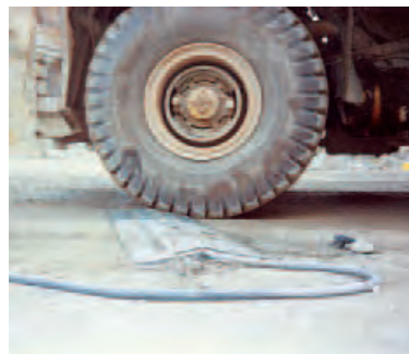
Trellex cable crossings.
