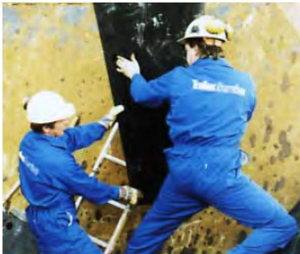
Truck type Cat lined with Trellex wear resistant elements type PP.
